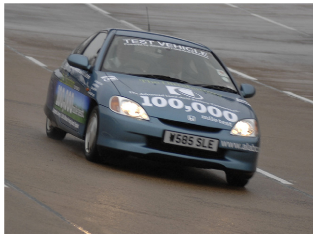
Fig. 3. Honda Insight with an 'Ultra' VRLA battery in place of the original nickel metal hydride battery completed over 100,000 miles with no conditioning or equalization and without failing.
